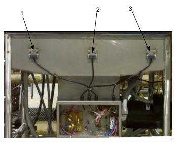
Front of rack conveyor showing the conveyor switches
